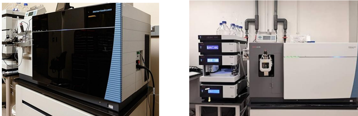
Figure 2. Ultrahigh-resolution Orbitrap Fusion Lumos 1M and Orbitrap IQ-X 1M mass spectrometers for the molecular and isotopic analysis of DOM.
